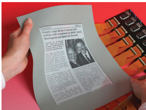
Fig. 7 Flexible active matrix display using e-ink Imaging Film. Printed with permission from Plastic Logic.
